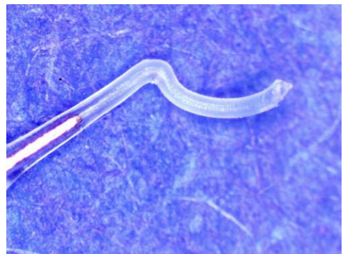
Figure 3. Microscopic image of a broken wire for case 8 (Z4) showing no arcing.
